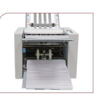
✓ Output conveyor with adjustable stacker wheels for neat, sequential stacking
