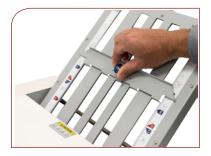
Clearly marked folds plates make setup a breeze
