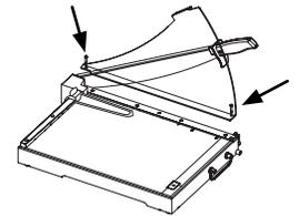
3. Raise the blade, insert paper, and adjust the side guide to the desired location.
