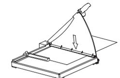
5. Lower the blade in a slow, steady motion to cut the paper.
