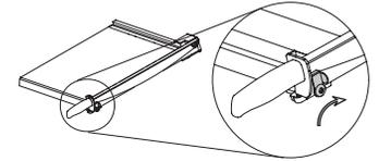
2. Carefully insert the safety shield. With the safety shield in place, lower the handle, and insert the 2 screws to secure the shield. (Be sure it is securely attached prior to use)
